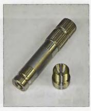
Cincom M32s in a cycle time of 72 seconds. This has been cut to 53 seconds, representing a 26% saving. With 55,000-off needed, the economy gained is significant.
